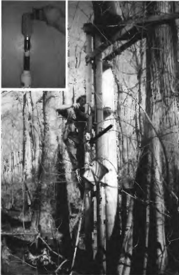
Figure 13.6. Example of an automated, single purpose water level recorder, the WL-80 being downloaded. The WL-80 (arrow) is mounted next to the stilling well of a Stevens type recorder. Inset shows the head of the WL-80 and the calculator used for downloading.
