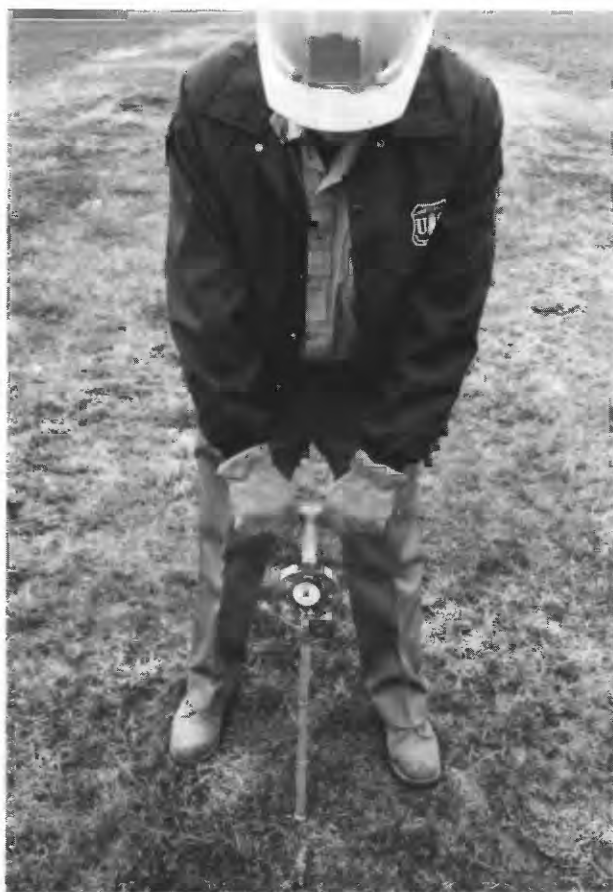
Figure 3.3. Soil penetrometer being used to assess soil compaction.
