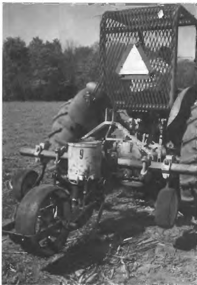
Figure 7.3. Two types of modified agricultural planters used for direct seeding: (a) planter requiring personnel to drop seeds in manually and (b) planter that drops seeds in automatically.
