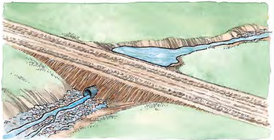
This temporary stream crossing culvert is too small. The stream is ponding behind the culvert and seeping through the fill. The culvert could fail, sending fill soil downstream.
