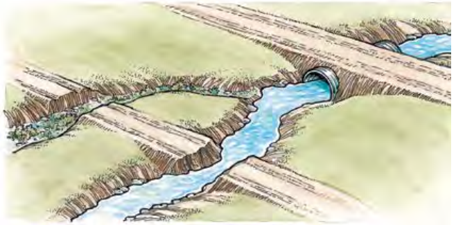
In this example, a minor relocation of the road prism resulted in only one culvert installed for road access. This reduces maintenance and allows the side channel below the new crossing to be restored to a more natural condition.
