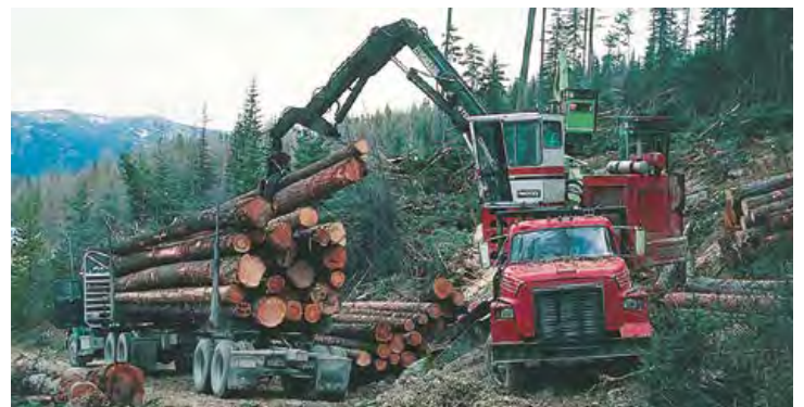
Left: Skidders or dozers drag logs from the forest to the log landing. To reduce soil disturbance, rubber-tired skidders or crawler tractors are kept on skid trails. Winch line and chokers pull logs to the machine. Right: At the landing, a log loader moves logs onto trucks for delivery to the mill.
